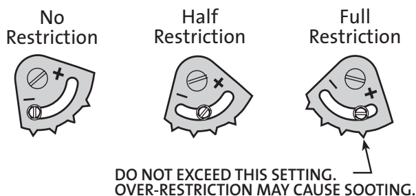
Figure 15. Exhaust Restrictor settings
